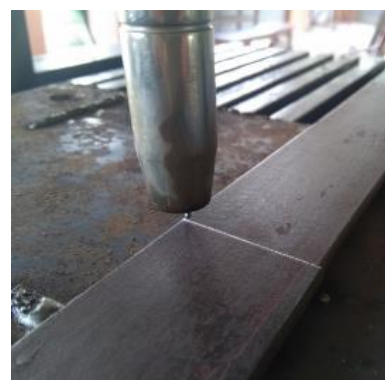
Figure 3. Gap between Base Plate and Tip of Welding Torch
